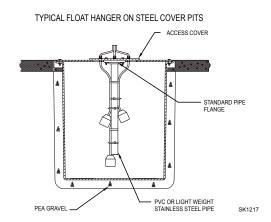
On some installations it may be desirable to install an independent hanger for the level control switches to avoid possible hang ups on the pumps, piping, valves, etc. Float hangers are available from Zoeller Company on Catalog Sheet FM0526 or can be fabricated from standard pipe and fittings.
