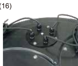
(16) Screw down the float tree plate.
