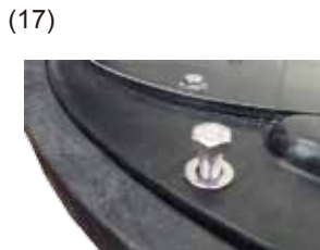
Align the cover and screw in tightly.
