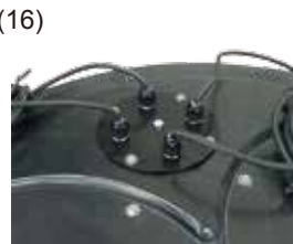
Screw down the float tree plate.
