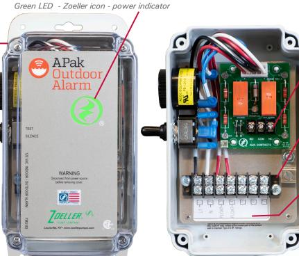
Auxiliary output for connection to additional alarm equipment, such as Z Control® Gateway. 5 amps max, 120 VAC.
